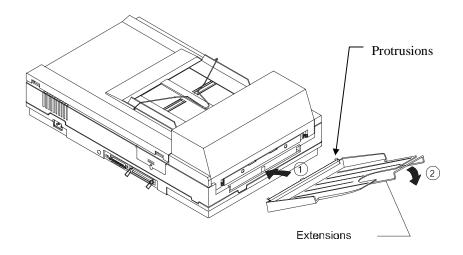
Figure 2-5 Install the ADF Output Paper Tray
